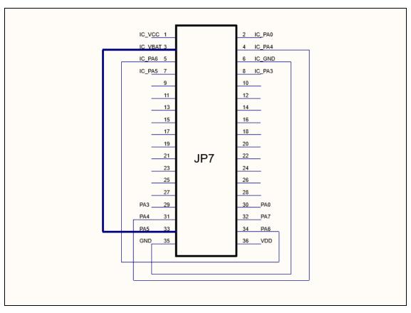
schematic diagram of Jumper7 for P003
